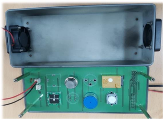
Fig.1 Atmospheric environment Sensing Device
