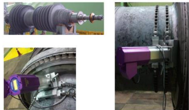
Fig.2 Measuring tensile strength of thermoelectric power plant
