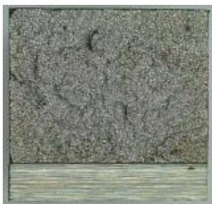
Fig. 5. Fracture surface of Charpy specimen at -50\text{ }^{\circ}\text{C} .
