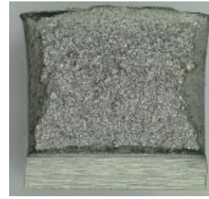
Fig. 6. Fracture surface of Charpy specimen at +20\text{ }^{\circ}\text{C} .
