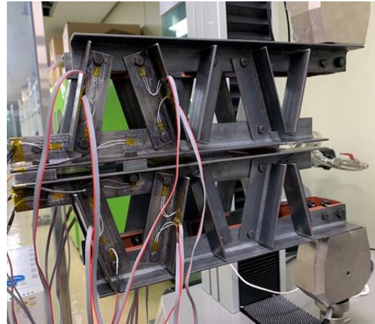
Fig.1 Truss model assembled with steel angles
