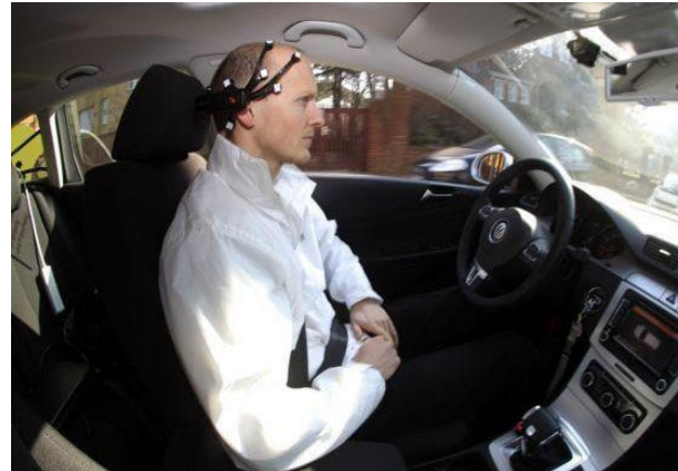
Fig.1 The example of the EEG signal acquisition in the automated vehicle
