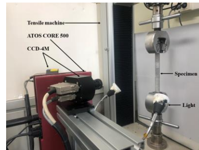
Fig. 1. The multi DIC system for specimen with hole in tensile test
