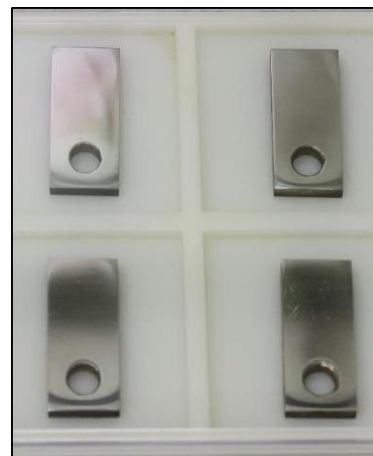
Figure 1. specimens used in this study. Upper ones are A106 Gr. B and lower ones are A335 P22 specimens every specimen was polished before experiment.
