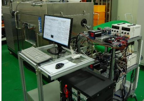
Fig. 4 BLDC motor operational ALT test apparatus
