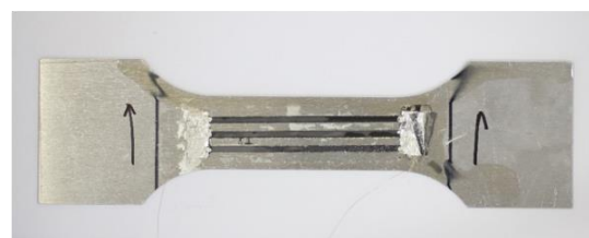
Fig. 2 Specimen design: ISO 6892-1 specimen dimension (top), SUS 304 specimen with sensing elements (bottom).
