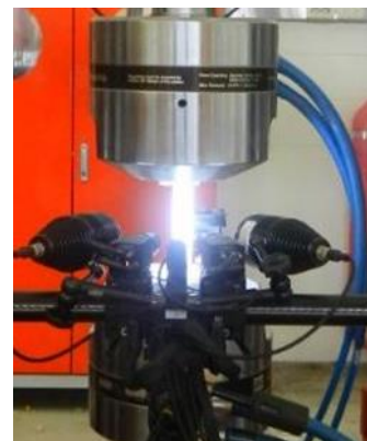
Fig.1 Experimental setup for cyclic fatigue load test and DIC measurement
