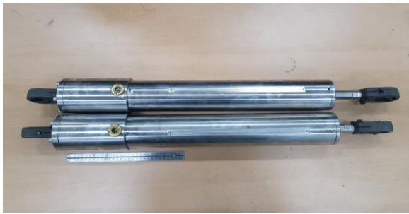
Fig.2 Hydraulic snubbers for accelerated aging test
