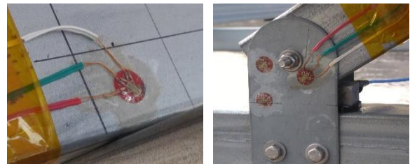
Fig.5 strain gauge installed on steel structure
