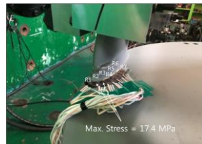
(b) Measured stress (equivalent one-point loading (5.244 kN))
