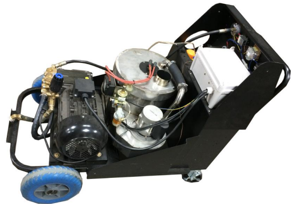
Fig.1 High-temperature high-pressure washer equipped with a waste heat recovery system
