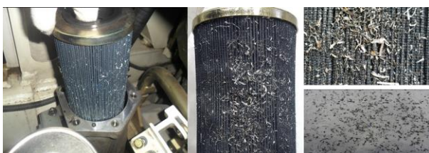
Fig. 1 Unidentified metallic foreign substances observed during annual maintenance
