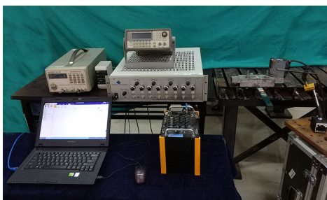
Fig. 1 Test set up for MFC actuation function degradation test
