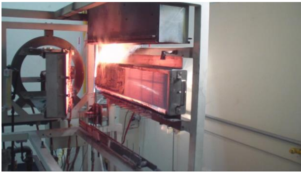
Fig.2 Reaction to fire test-spread of flame
